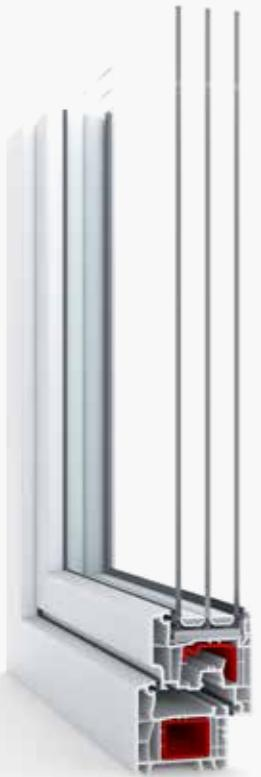
In a configuration with the new half-recessed sash, with the option of glazing with glazing units up to 48 mm wide, it is possible to create even warmer window constructions in the IDEAL 4000 system (up to  $U_w = 0.85 \text{ W/m}^2\text{K}$ ).
